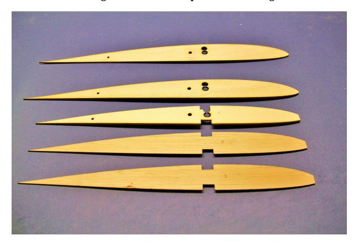
The top two parts are plywood, one is used as a root cap to the wing, the other is placed on the outside of the fuse.
