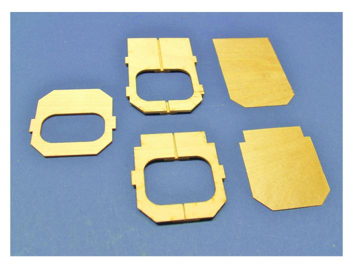
Modified formers # 1 and 2 to width of former #3 to reduce frontal drag. This means the wing root will be squared as opposed to the angle on the plan. I ran the two formers through the saw, carefully glued plywood supports to one side to insure they match the width of #3. Cut to fit 1/64" ply to be applied to front sides of #1 and 2 to hide the saw cuts.
