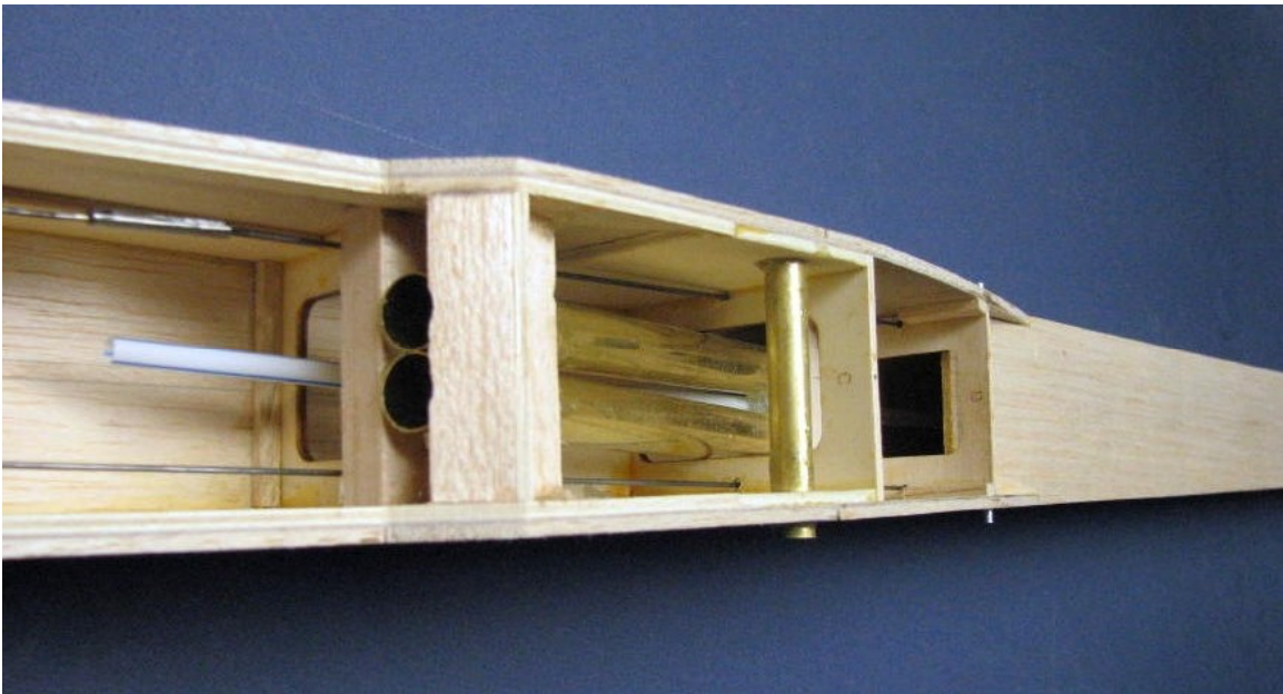
Tin foil used to protect the wood from solder iron when installing a push rod coupler joining the push wires together. Large clamp is holding wire in position while soldering coupler. I pre-heat the coupler.
